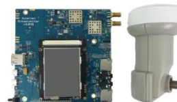
Included antenna: Maverick MK1-PPL approx. 3.8" x 2.5" (shown to scale)
