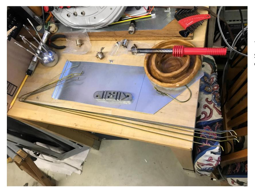
Cut off hooks and straightened hangers with help of bending jig. - calculated that 23" would be more than enough length for 445.mHz (20-ish in. for .25 wl)
