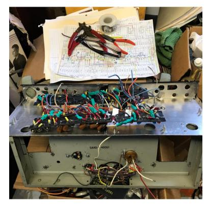
Circuit boards were kept intact. Holes cut & drilled into the chassis.
